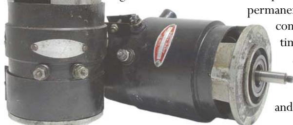
heavy, weighing between 9.25 lbs (Delco-Remy 1101876) and 15.4 lbs (Delco-Remy 1101898). In addition to sheer weight, these units also have the disadvantage of requiring frequent maintenance—often due to worn brushes or commutators.
