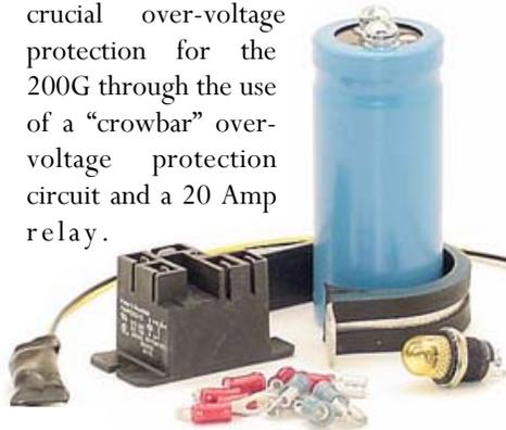
Each kit also contains a clear-yellow warning light that will illuminate if the OV protection circuit has been “tripped” (or when the alternator switch has been left off), and a filter capacitor to reduce radio noise and enhance regulation.
