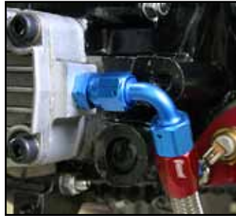
The oil line runs from the bottom of the Turbo body (left photo) to the left port of the secondary oil pump (right photo).
