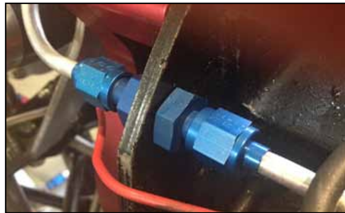
The bulkhead fitting installed through the engine case flange (fence baffle not shown in this photo).
