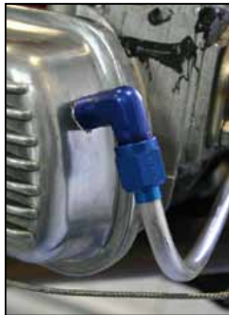
The oil line runs from the right port of the secondary oil pump to the valve cover.
