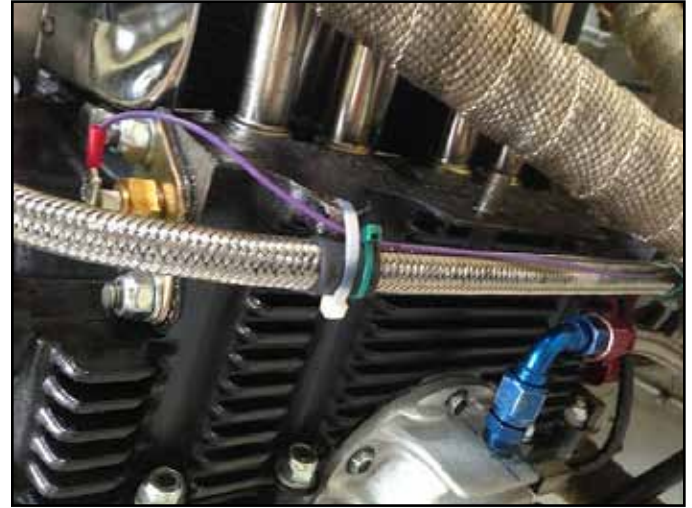
The oil line secured under the engine case.
