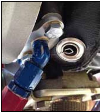
The oil line runs from the bottom of the Turbo body (left photo) to the left port of the secondary oil pump (right photo).
