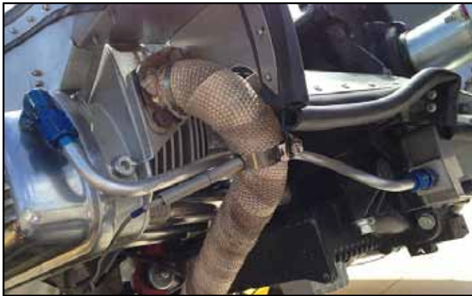
The oil line runs from the right port of the secondary oil pump to the valve cover.
