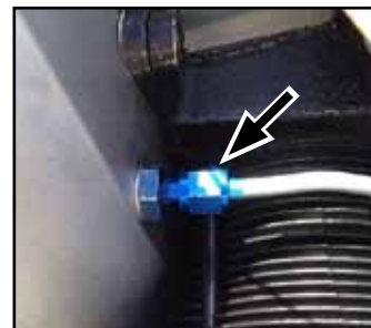
Looking down on the bulkhead fitting installed through the engine case flange and rear fence baffle.
