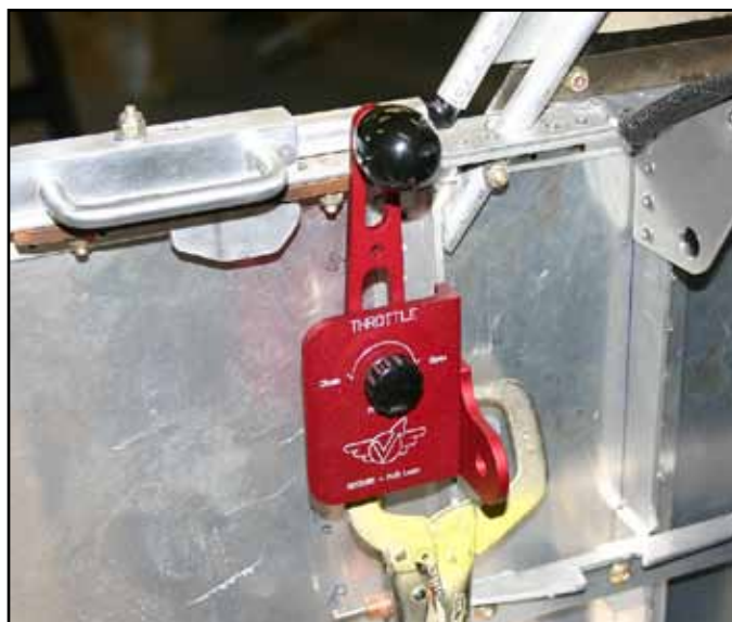
The throttle quadrant is clamped in place prior to drilling the mounting holes. Note that this aircraft needs to have the forward canopy handle moved aft to eliminate interference with the throttle quadrant.
