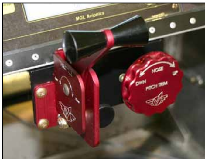
This center-mounted quadrant is attached to a 1/8" thick angle extrusion mounted under the panel.
